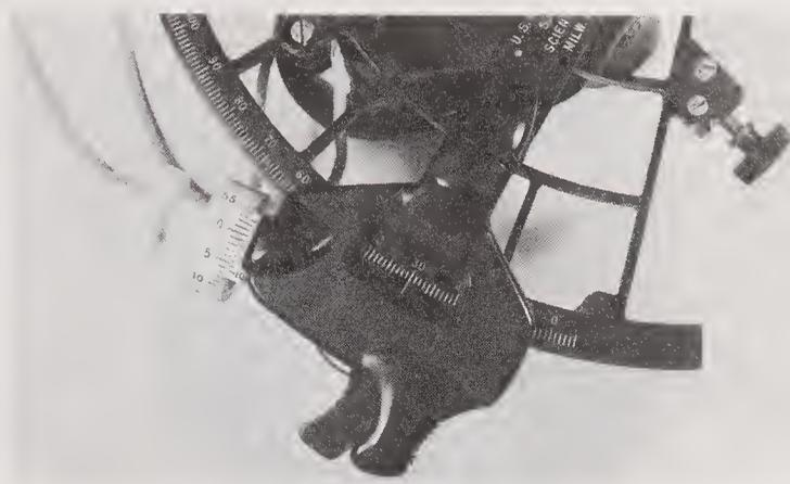
Figure 2106b. A U.S. Navy sextant showing the index mark opposite the 30° mark. The correct angle is 29°57' and not 30°57'.
