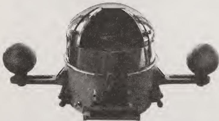
Figure 309a. U.S. Navy standard No. 3, 5-inch alcohol-filled compass in binnacle.
