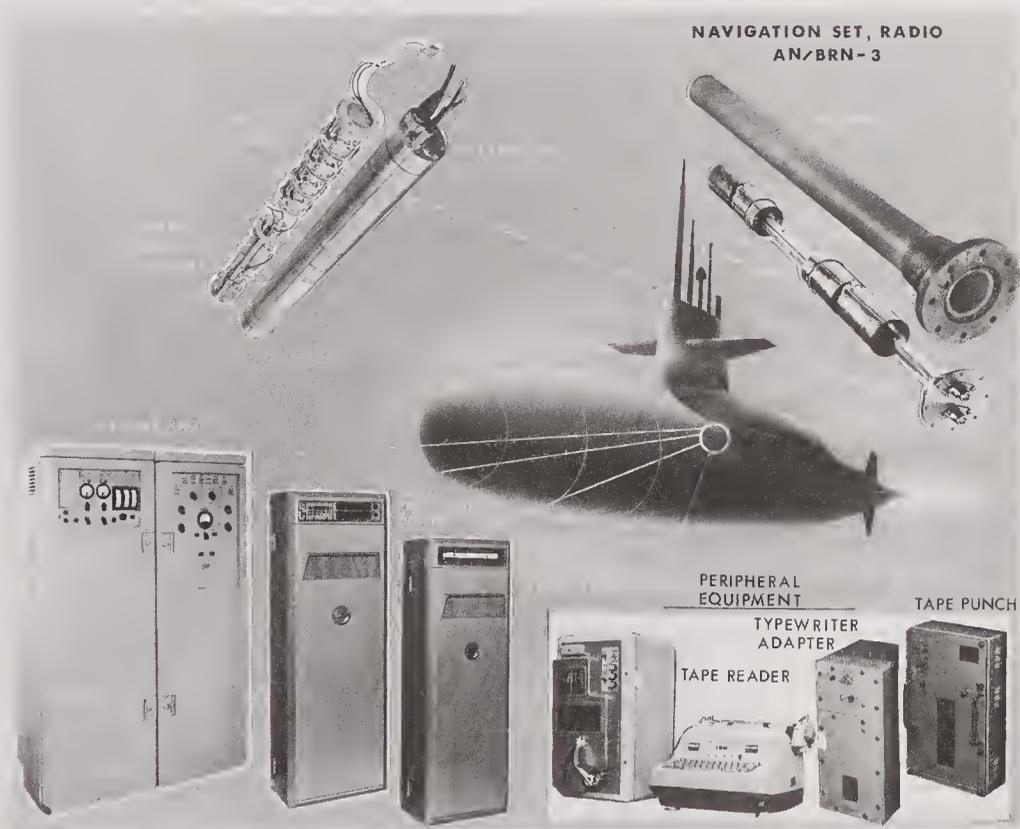
Figure 3408b. AN/BRN-3 equipment for submarine use of satellite navigation.
