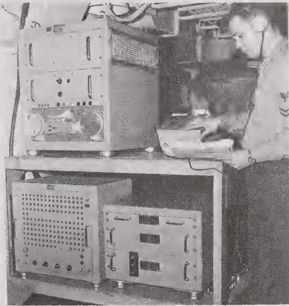
Figure 3408a. AN/SRN-9 shipboard receiver for satellite navigation.
