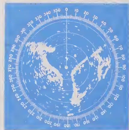
Figure 1602c. Radar PPI display.
