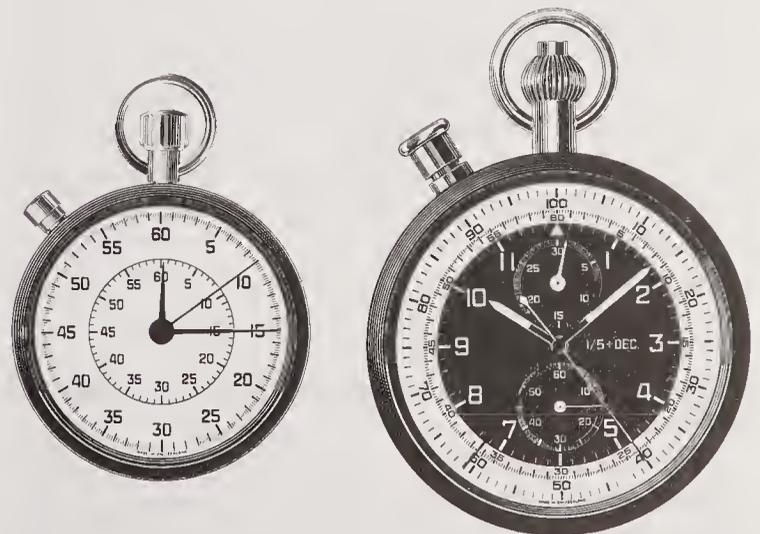
Figure 727. A stopwatch (left) and a chronograph with split-second capability.
