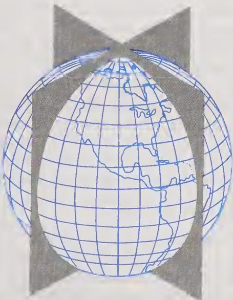
Figure 204c. Meridians of longitude are formed by planes that contain the earth's axis.
