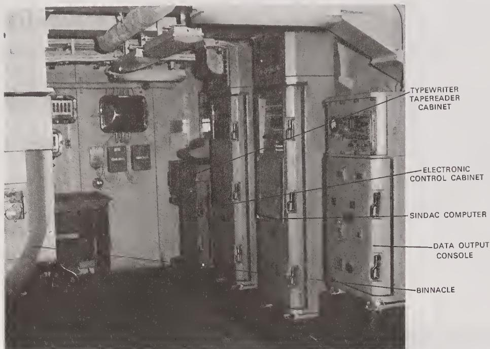
Figure 3507c. Mark 3, Mod. 5 Ship's Inertial Navigation System (SINS).
