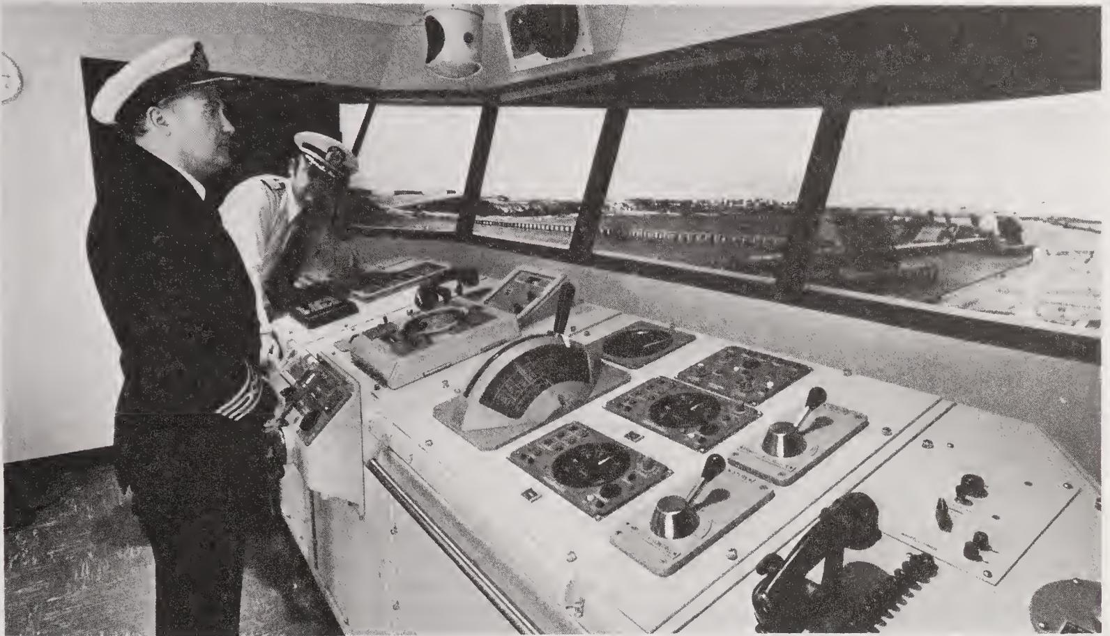
Figure 1511. A typical merchant ship pilothouse equipment installation reflects the much smaller manning level of this type of vessel, compared with the naval ship.
