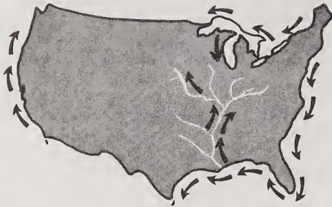
Figure 405a. Direction of increasing numbers for coastal buoys—as if “returning from sea.”
