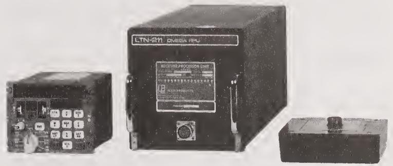
Figure 3309a. Omega Navigation System receiver as used aboard U.S. naval vessels.
