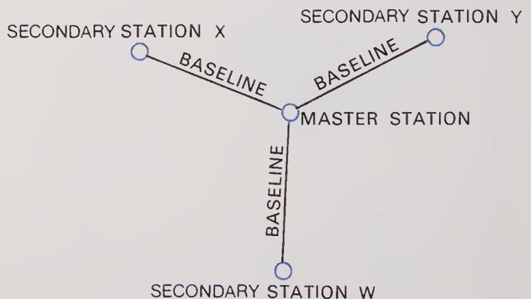
Figure 3216a. Loran-C "star" configuration of one master and three secondary stations.
