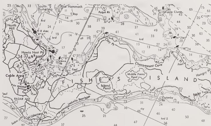
Figure 529. Vertical lettering is used for features that are dry at high water; slant letters for submerged and floating features.
